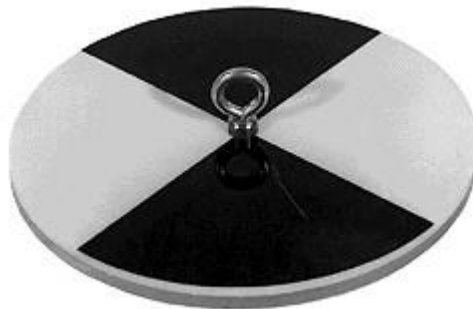
Figure 4. A Secchi Disc is a method to assessing the clarity of water in lakes and ponds. Secchi measurements are made in the shade with the sun to your back to make an accurate and reproducible reading.
