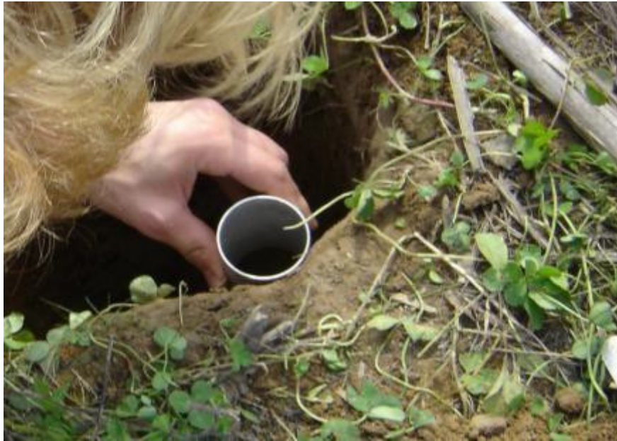
Figure 12: A metal core is used to collect soil core sample for bulk density measurements (University of Rhode Island, n.d)
