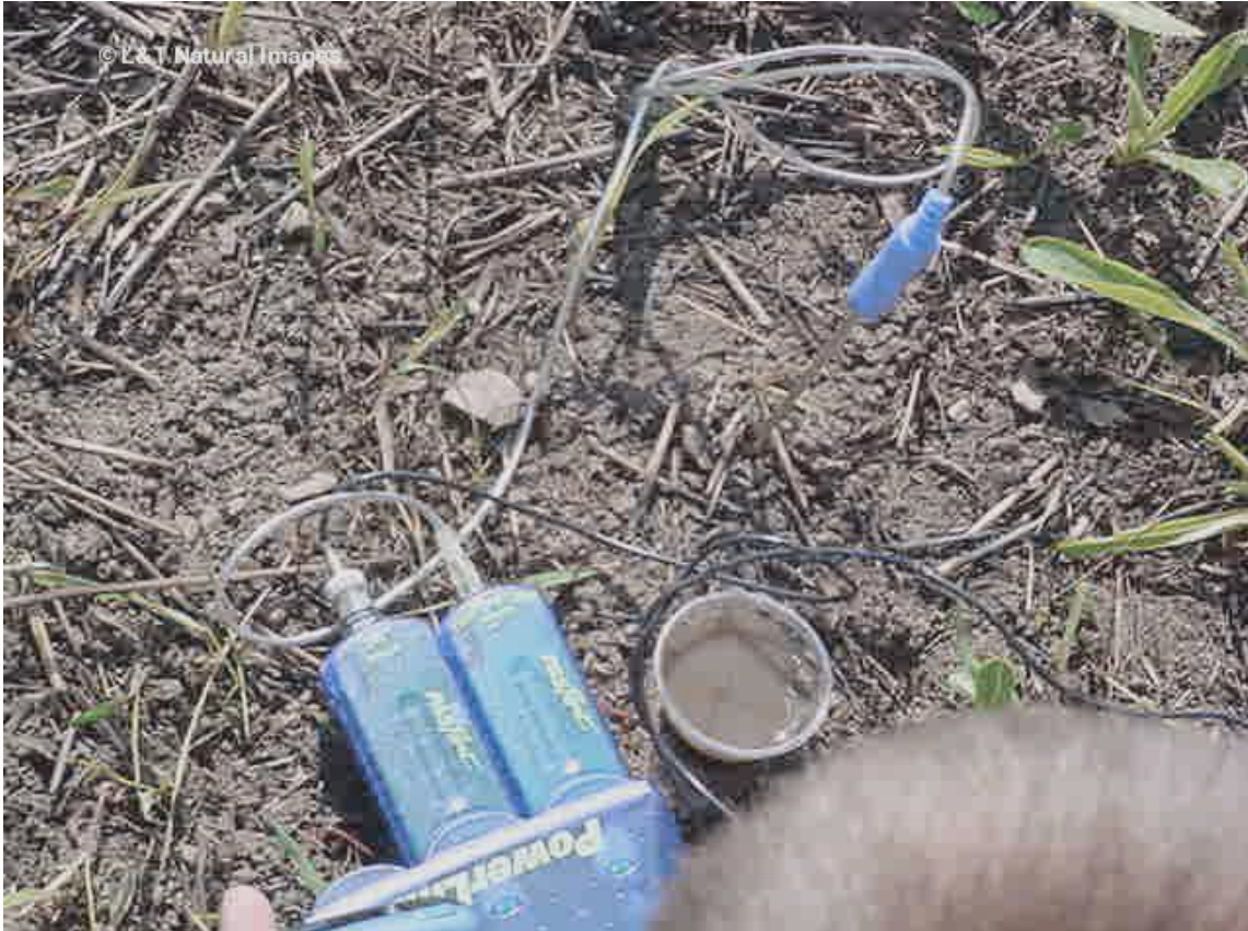
Figure 15: A soil temperature probe can be used to measure the temperature of the soil at various depths ( http://www.ncusd203.org/madison/Links/teams/training.html )
